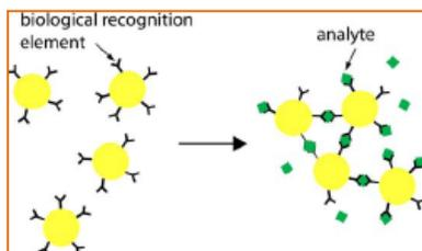
Schematic representation of a colloidal biosensor
