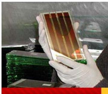
**Figure 4.** A dye solar cell (DSC) commercialised by DyeSol (source: [www.dyesol.com](http://www.dyesol.com))
