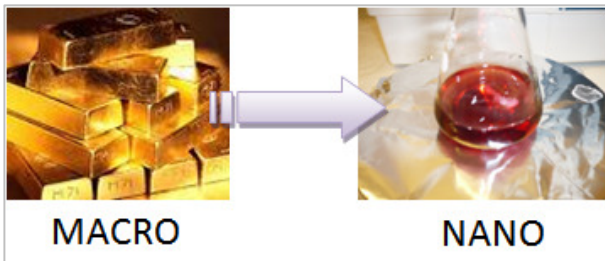
Figure 1. Dependence of colour on gold size. (Image source: L. Filippini, iNANO, Aarhus University, Creative Commons ShareAlike 3.0)
