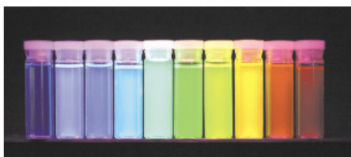
Figure 11. Ten distinguishable emission colours of ZnS-capped CdSe QDs excited with a near-UV lamp. (Reprinted by permission of Macmillan Publishers from Macmillan Publishers Ltd: Nature Biotech. (2001) 19, 631-5, Copyright 2001).
