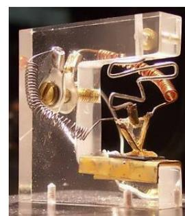
**Figure 1.** Replica of the first bipolar Transistor. This replica was photographed at the Nixdorf-Museum, Paderborn, Germany. (Image credit: Wiki Commons, Creative Commons Attribution ShareAlike 3.0)
