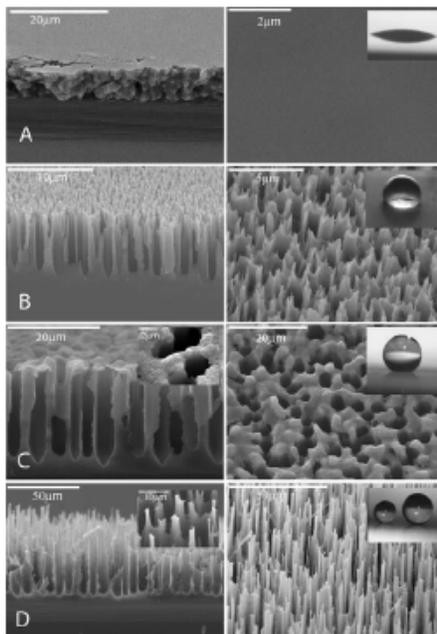
**Figure d10.** SEM Images of four different samples showing a change in contact angle from hydrophilic (A) to hydrophobic and superhydrophobic. Samples B-D are made of porous silicon, sample D is the one with the higher contact angle (Image reprinted with permission from: A. Ressine, "Development of protein microarray chip technology", PhD thesis 2005)
