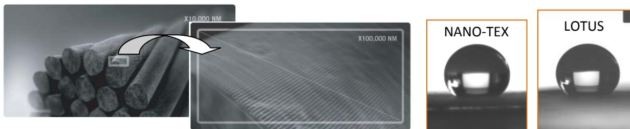
**Figure 8.** Left: High resolution images of the Nano-Tex® fabric (Images courtesy of Nano-Tex, Inc., Copyright Nano-Tex. Inc). Right: contact angle images of water droplets on Nano-Tex fabric and Lotus leaf (Images: iNANO; Aarhus University, Creative Commons Attribution ShareAlike 3.0).
