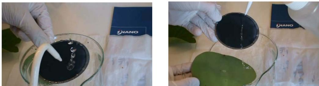
**Figure 9.** Images from NANOYOU Video 4-“Lotus Effect-Part 2” showing the wetting properties of a piece of porous silicon (left) and how this material compares with a real lotus leaf (right). (Image credit: iNANO, Aarhus University, Creative Commons Attribution ShareAlike 3.0)
