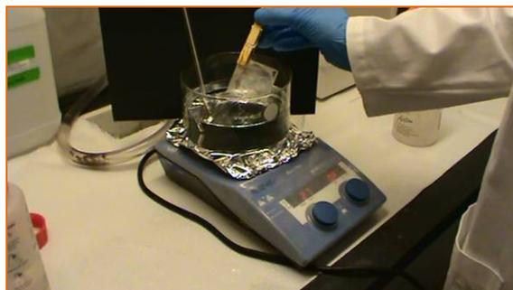
Hold the first liquid crystal Sheet 1(type 1) with a clothes peg and immerse it the water bath (see figure below). Do you see any colour? Now increase the hotplate temperature so that the water reaches 23° C. Record the colours that you see as the temperature increases:
