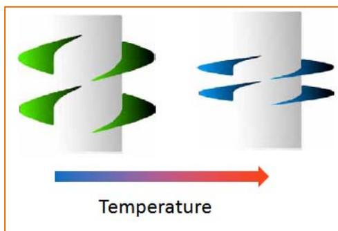
**Figure 5.** Representation of a pitch change in a chiral LC as the temperature is changed. (Image credit: Image adapted from IPSE Educational Resources (Liquid crystals), University of Wisconsin Madison).
