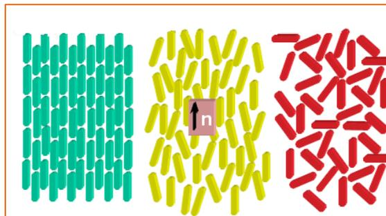
**Figure 1.** Schematic representation of molecules in a solid (left: molecules are well organised); in a liquid crystal (centre: molecules have a long range distance order) and in a liquid (right: molecules are not ordered). (Image credit: Copyright IPSE Educational Resources, University of Wisconsin Madison)
