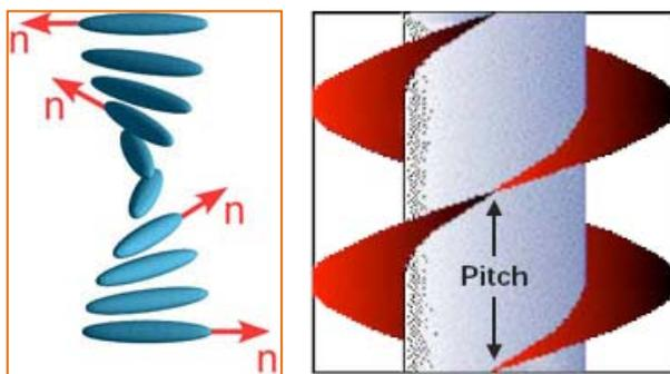
**Figure 4 (Left):** Schematic representations of stacked rotating layers in a chiral LC forming a “spiral staircase” having a pitch  $p$ . (Right) schematic representation of the pitch in a chiral LC. Images credit: Wiki Commons, Creative Commons Attribution ShareAlike 3.0)
