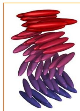
**Figure 3.** Schematic representation of ordering in chiral liquid crystal phases: a chiral nematic phase (also called the cholesteric phase) in an LC (Image credit: Wiki Commons, Creative Commons Attribution ShareAlike 3.0).
