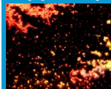
An optical microscope image of gold nanoshells deposited on a glass microscope slide. (G.Koeling, University of Wisconsin-Madison NISE Network, www.nisenet.org, licensed under NISE network terms and conditions).
