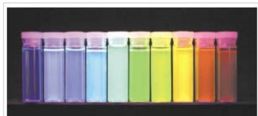
**Figure 13.** Ten distinguishable emission colours of ZnS-capped CdSe QDs excited with a near-UV lamp. From left to right (blue to red), the emission maxima are located at 443, 473, 481, 500, 518, 543, 565, 587, 610, and 655 nm. (Reprinted by permission of Macmillan Publishers from Macmillan Publishers Ltd: Nature Biotech. (2001) 19, 631-35, Copyright 2001).
